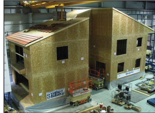
A full-size townhouse, shown here almost completed, was built on a “chassis” spanning between the two tables and tested to simulate an earthquake.
