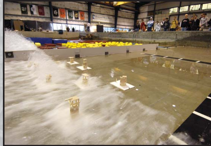
Tsunami simulation with scale-model structures in the Oregon State University tsunami wave basin.
