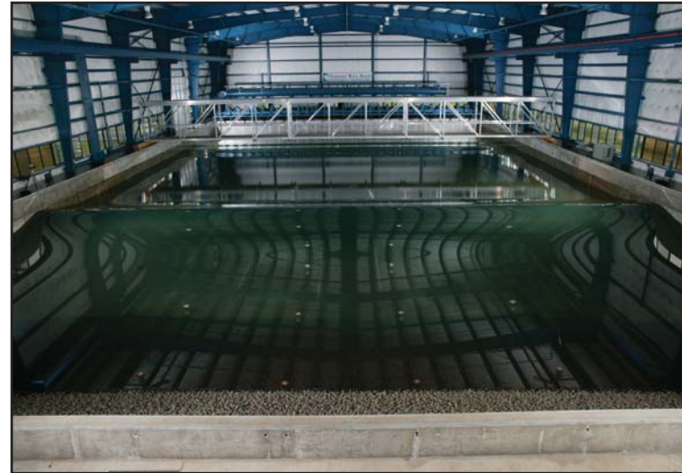
The tsunami wave basin has piston-powered hinged paddles that generate precise shapes and sizes of waves.
