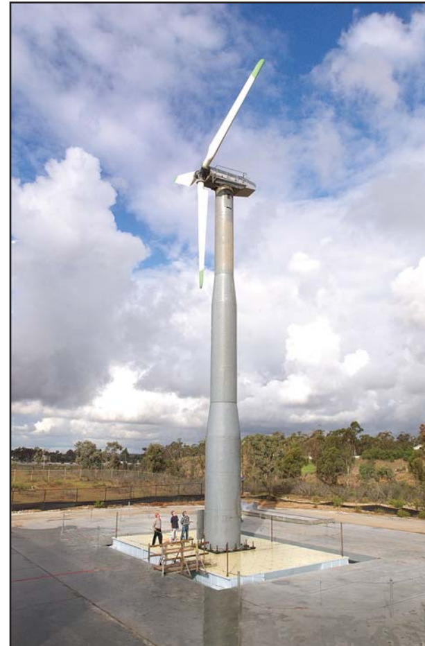
An actual wind turbine, 21 m (70 ft) tall, has been tested on the outdoor UC San Diego shake table.
