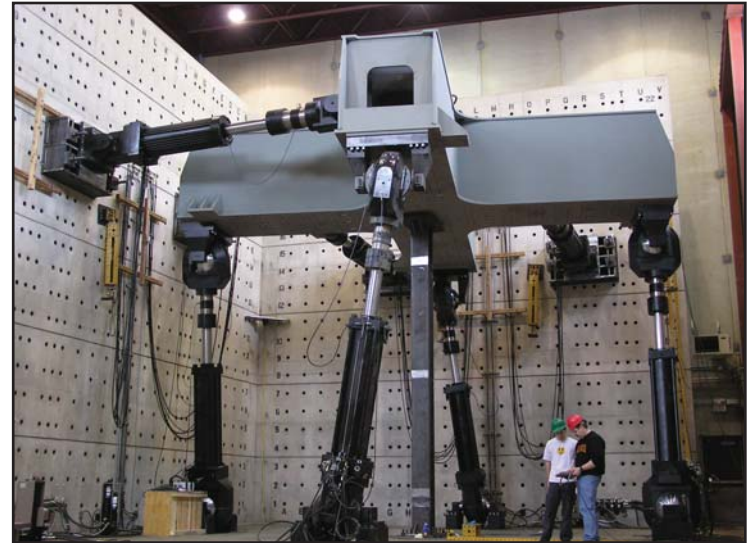
The steel box column mounted in the center of the apparatus at the University of Minnesota is experiencing a simulation of the earthquake motion of the structure above it.
