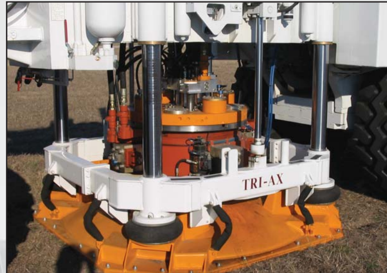
A vehicle-mounted vibrating machine that can simulate earthquake motions is shown with its plate firmly in contact with the ground, ready to begin a geotechnical engineering test.
