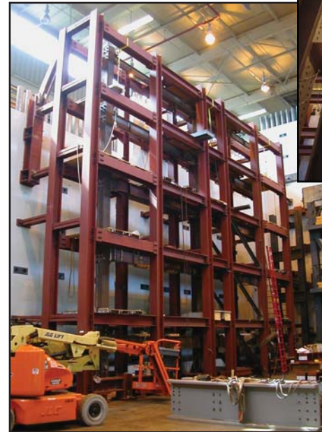
Full-scale buildings several stories high are subjected to seismic simulations in the research site at Lehigh University.
