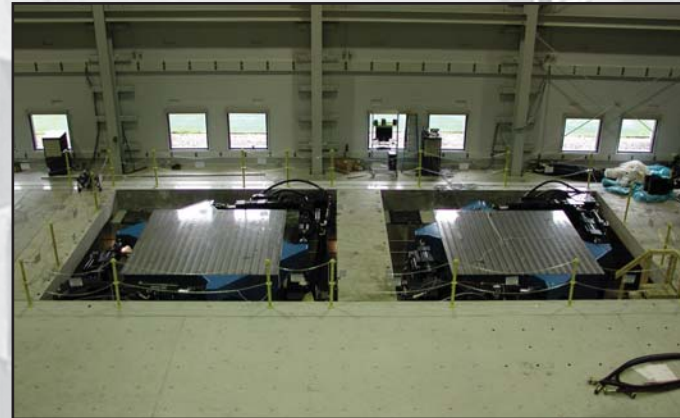
One of the NEES facilities at the University at Buffalo has two tables that can be used independently or with a framework spanning between them to provide a larger "footprint."
