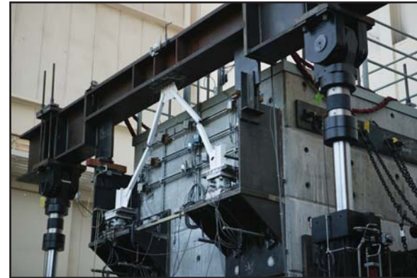
A test in the UC Berkeley NEES facility of a portion of a braced frame.
