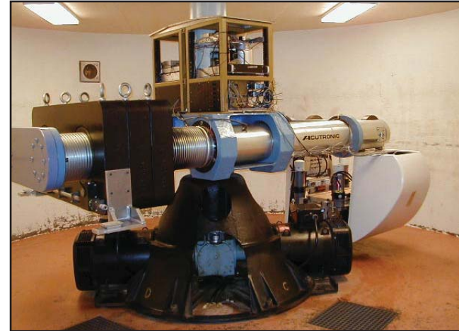
The geotechnical centrifuge at RPI; at left the counterweight, at right the hinged container for the soil to be modeled (which swings into a horizontal position during operation).
