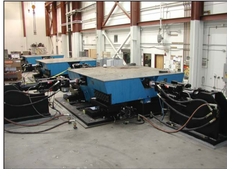
The three biaxial shake tables at the University of Nevada, Reno laboratory.
